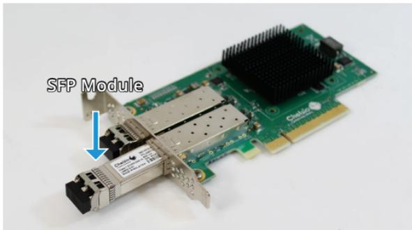
The SFP+ module has a rubber dust cover. Keep the cover in place until ready to connect a fiber optic cable. To remove the dust cover, lift the handle until it is fully open and pull the dust cover off.
