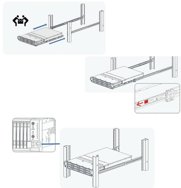
To remove the TrueNAS Array, remove securing screws, fully extend the unit until it is in the locked position, and pull the pin lock latches to release the lock. Now remove the unit from the rack. To remove the inner rails from the TrueNAS Array, remove all securing screws and slide the rail as indicated to release from the system chassis.
