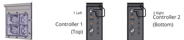
**Note:** The power button on the left side of the TrueNAS Array corresponds with Storage Controller 1 (top) and the power button on the right corresponds with Storage Controller 2 (bottom). In non-HA systems, the buttons for Storage Controller 2 are disabled.
