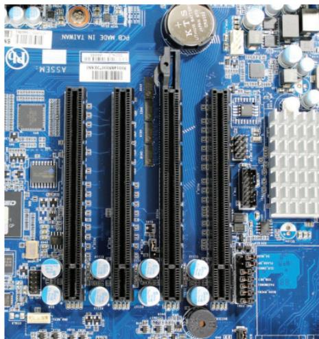
Align the four edge connectors with the PCIe slots on the motherboard. Press down evenly on the PCIe Bus Riser until the edge connectors click into place and are firmly seated.
