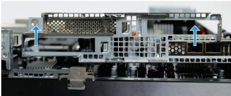
Locate the PCIe Bus Riser release latch. Press on the release latch while lifting the PCIe Bus Riser to remove it completely.
