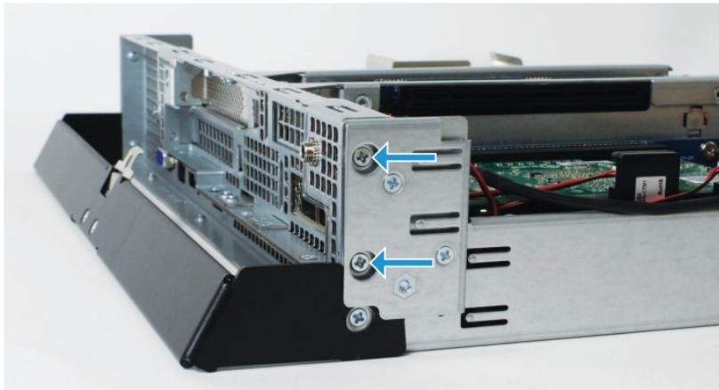
Replace the second slot cover retainer and the two screws.
