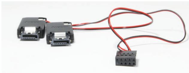
Align the SATADOMs with the **SATA\_3** and **SATA\_5** slots on the motherboard. Press down until each connector clicks into place. The USB header connector is connected to the **Front\_USB** header on the motherboard. Make sure the red wires are on the right-hand side of the connector, line up the pins with the connector, and gently press down until the connector is fully seated.
