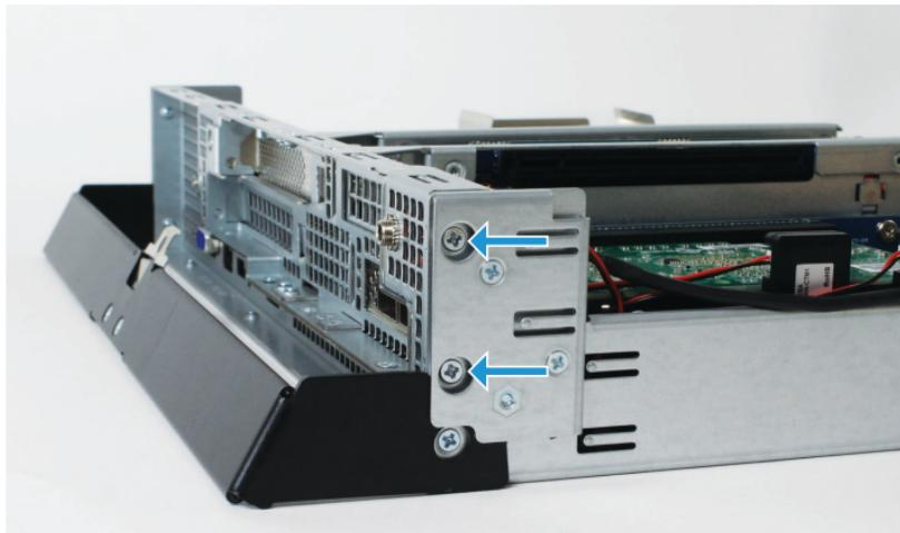
Place the slot cover retainer next to the node with the wires still attached.
