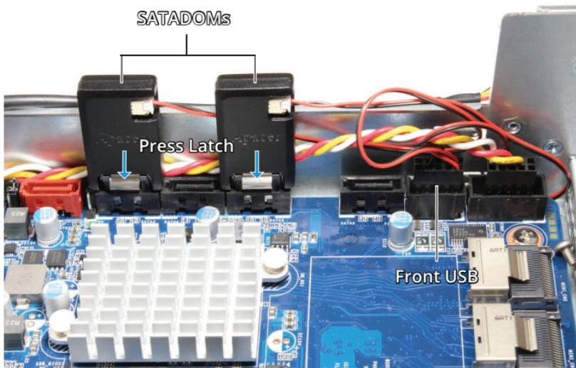
Both SATADOMs are powered from one cable attached to the **Front\_USB** header on the motherboard. Use thumb and index finger to grip the USB power connector and gently pull upward to disconnect.
