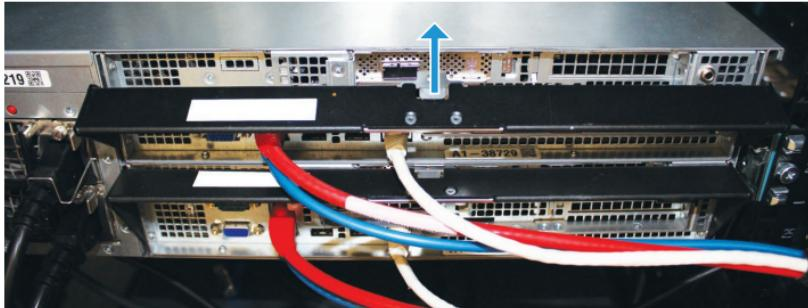
Reconnect the network cables to the node. On a single-node non-HA system, also plug in the power cable and power on the system.
