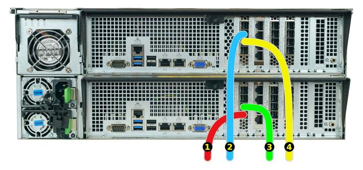
Connect SAS cables to the ES12 T slots. These are the typical SAS connections for one or two ES12 expansion shelves connecting to a High Availability (HA) TrueNAS® system with two storage controllers. When a TrueNAS® unit with only a single storage controller is used, only cables #1 and #3 are connected.
