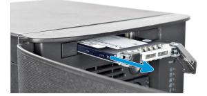
To add an SSD, unscrew the two attachment screws from the SSD tray underside and remove the SSD tray filler. Attach the cache SSD to the tray with four screws from the bag labeled 2.5" through the bottom of the tray.
