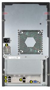
Both systems have back-panel power connectors (1), VGA video connectors (4), and IPMI remote management network ports (6).
