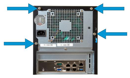
Slide the black metal cover off the back of the chassis by lifting the blue retention lever, grasping the sides, and pushing the cover and chassis back panel apart. When the cover can no longer move away from chassis frame, gently lift the cover up and away from the chassis frame.
