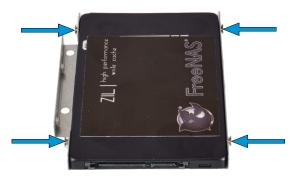
Replace the tray on the chassis by aligning the tray retention clips with the holes in the chassis, sliding the tray into place, and reattaching the original screws. Repeat the process if a second SSD is being installed.
