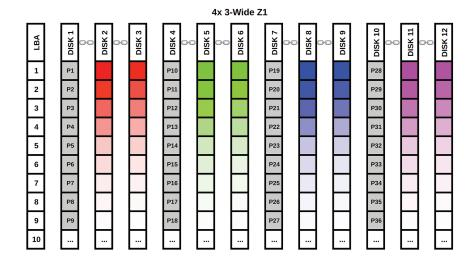
Each stripe gets its own parity sector, but unlike the previous examples, we only have a single parity sector per data stripe. This is why RAIDZ1 is not highly fault tolerant and is thus not a recommended configuration for storing mission-critical data.
