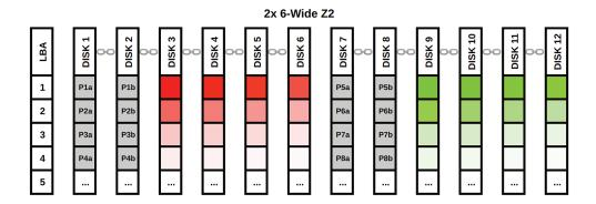
As in the Z3 diagram, each data stripe gets its own pair of unique parity sectors. The first data block is written to the first vdev and the second data block is written to the second vdev. A third data block would again be written to the first vdev, and so on.
